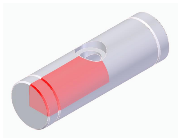
Figure 11. CEM FP cavity model with the simulated section dyed in red.
